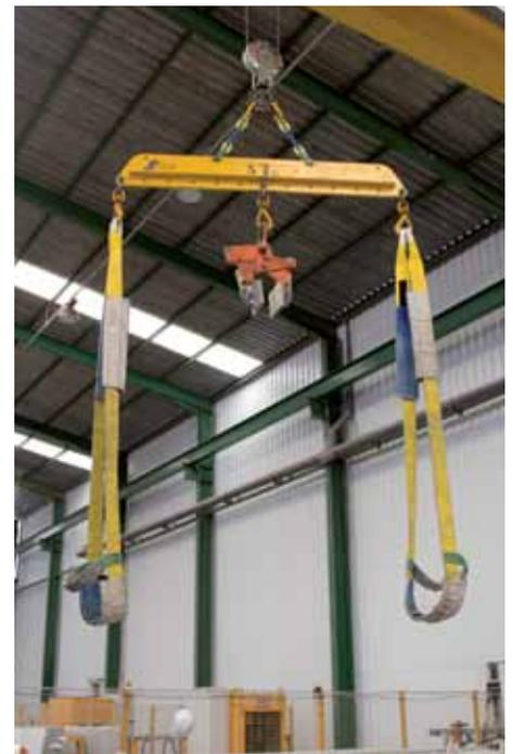
When positioning DEKTON® slabs on racks, take extreme care to prevent breaking the edge of the material.
